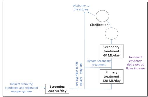
suspended solids and treat pathogens from the combined system and, while has some benefits for reducing nutrient levels in effluent, it is not its primary purpose. The following figure shows how Ti Tree Bend functions.
