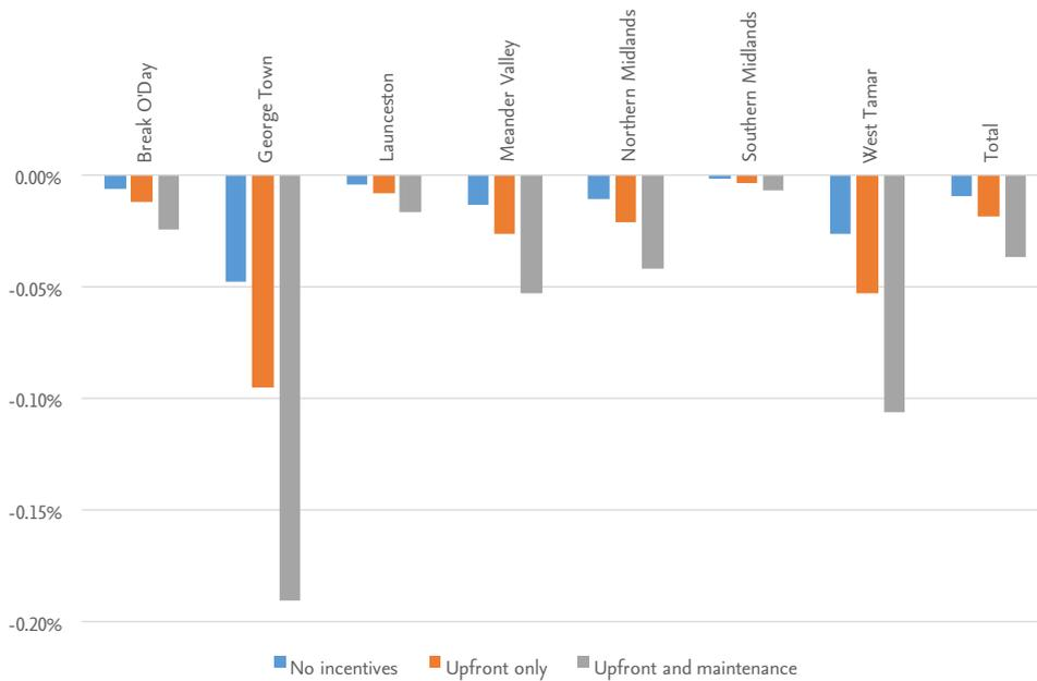
Figure 37. Modelled impact of large scale water sensitive urban design option scenarios on diffuse plus combined sewer overflow pollutant loads
