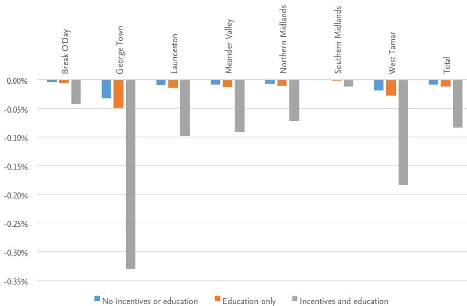
**Figure 38. Modelled Impact of household scale water sensitive urban design option scenarios on diffuse plus combined sewer overflow pollutant loads**
