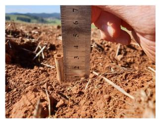
Loss of soil was measured at the Deloraine trial site using a series of bamboo sticks.
